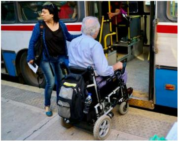
Otherwise accessible buses may have overly large horizontal or vertical gaps that stop passengers with disabilities from crossing from platform to bus floor.
