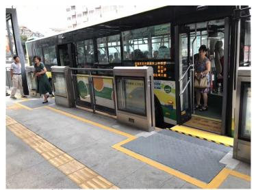
Gap filler deployed at Yichang BRT station
