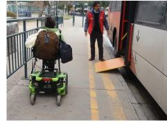
to the bus can easily be too steep if the stop is not high enough to permit safe deployment of the ramp at, ideally, no more than a 12% grade. (Compare photo above with the flat entry in the photo from Yichang at top left.) Ramps should have proper safety edges on their sides and should not have edges at either end which cannot be easily surmounted by the smaller wheels typically at the front of a wheelchair.
