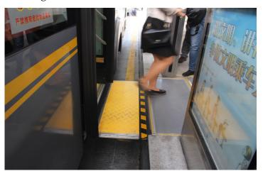
A movable bridge, deployed from the *platform* of this bus rapid transit station in Yichang, China, eliminates the station-to-bus gap for all passengers. If the bridge deploys *while* the bus doors are opening, travel time would not be effected. – ITDP photo forwarded by Gerhard Menckhoff
