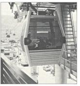
These systems are accessible to wheelchair users and other disabled persons because the gondola floor is level with station platforms. Gondolas go temporarily "off line" at stations, enabling passengers to board the stationary passenger cabin. Some cities have several cable lines with multiple stations. - Photo above taken by Tom Rickert in Medellín, Colombia, April 2005.
