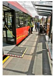
access including reduced gaps that wheelchair users can (usually) cross, or bridges to serve this purpose when needed, as shown in the photo at left on Line 5 through the citv's historic district. Also note the tactile guideways. Other features include good color contrast, priority seating, and improved audio and text signage.
