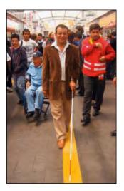
improvements include a deeply grooved tactile guideway to assist blind passengers (photo at left) and Braille information plates. Wheelchair users can access a button to operate a warning light to notify approaching bus drivers to carefully dock their buses to reduce the horizontal gap of some 10 cm between the raised station platform and the floor of the bus. However. much work
